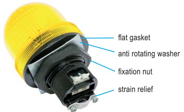
Easy bulb change due to rear access via bayonet detachable insert with BA15d socket for incandescent bulbs; clamping yoke terminal technique for high contact safety
