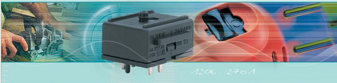
The double-sided lifting contact system of the 1206 series slide switch offers a robust and reliable solution as well as excellent electrical ratings. The 1206 series, which is suitable for both corded and battery applications, is distinguished by a superior rating of up to 8 (8) A 250V ~ 5E4, 15 A 125 V AC and 25 A 12-36 V DC.
