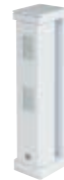
01740 Curtain-effect detector to protect entrances and openings such as doors, windows, covered terraces, corridors and French doors, short-range curtain-effect detection with adjustable lens up to 2 m or 5 m, PET immune, anti-masking function, 1 NO or NC 28 Vdc 0.1A relay output, surface mounting, 9.5-18 Vdc 20 mA power supply
