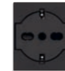
▲30211.G 16 A universal flush-fitting socket outlet, P40 - 2 modules Depth: 30,4 mm
