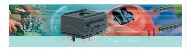
The double-sided lifting contact system of the 1206 series slide switch offers a robust and reliable solution as well as excellent electrical ratings. The 1206 series, which is suitable for both corded and battery applications, is distinguished by a superior rating of up to 8 (8) A 250V ~ 5E4, 15 A 125 V AC and 25 A 12-36 V DC.
